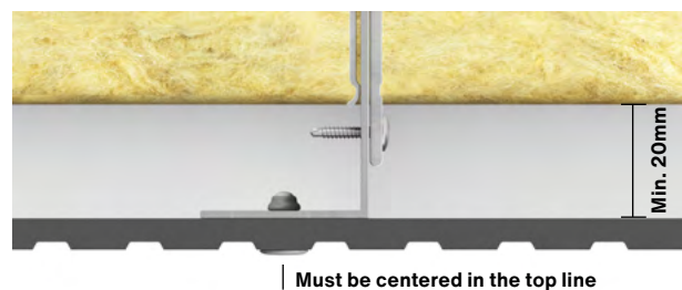
Fig. 2. Swisspearl Patina Inline installation on L profile.
